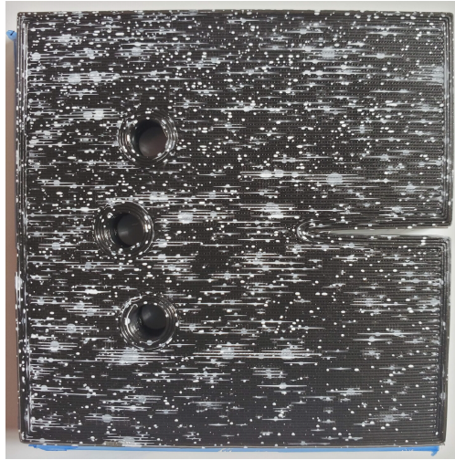
Figure 6: Spray painted speckle pattern used for digital image correlation (DIC).
